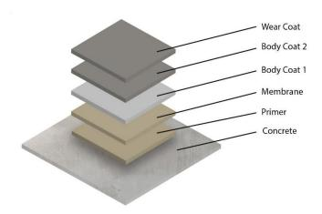
Install at manufacturer's recommended coverage rates and back roll thoroughly to endure pinhole free finish. Install a random broadcast of PCA 322 or PCA 323 aggregate into the wet primer to promote adhesion of next coat.
